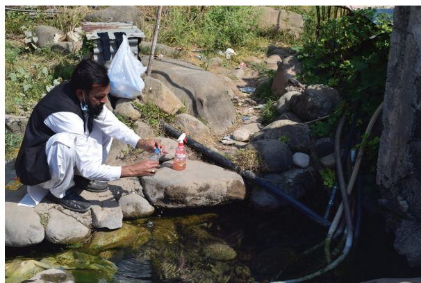
Figure 2. 3 Sampling and field chlorine testing of water sources
